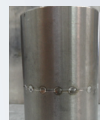
Pipe butt weld Ø 31.75 x 2 mm
